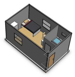
This Bedroom Module is used lightweight concrete for wall and roof. This module is reinforced by SHS 100 x 100 mm steel structure and it has flat roof, include bathroom inside.
